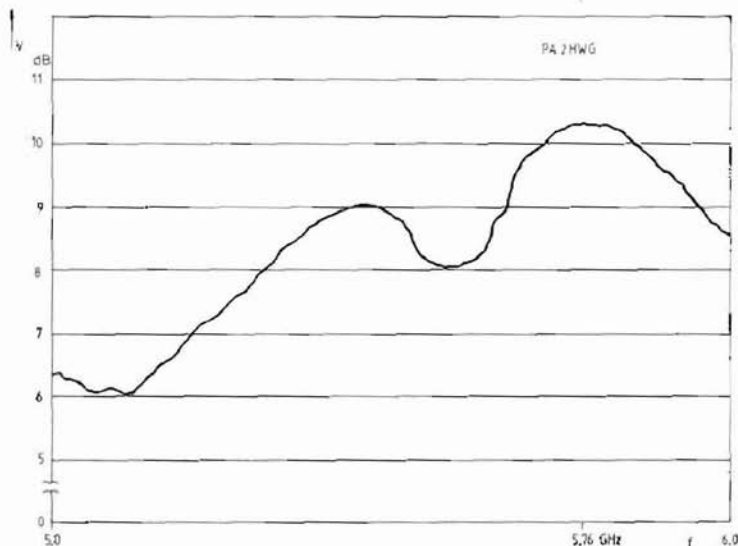
Fig. 5: The gain in the 6 cm amateur band amounts to approximately 10 dB.
